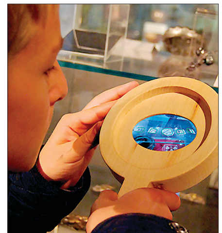
Figure 3. An example of a functional prototype using a newly repackaged mobile phone. In this example, an augmented-reality application on the phone is presented to the user as a magnifying glass.
